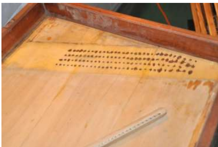
Wrestplank crown piece off, ready to re-apply towels to soundboard on top of wrestplank
