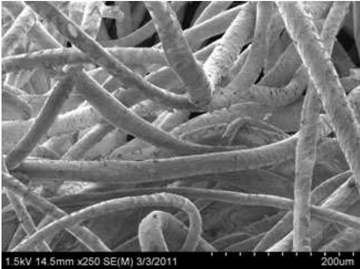
Wool, 1784 Broadwood, in scanning electron microscope at 250 and 700 X
