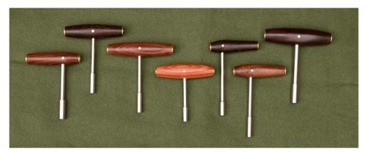
Obviously you need one, and it is important that it should be a good fit. Old instruments have hand-made flattened pins, and the hammer should grip the flats along the whole length (the ends do not matter). If the fit is sloppy, the corners of the pin will damage the socket, and be damaged themselves. There will also be backlash, which makes accurate tuning more difficult. On the other hand, if the socket is not big enough, it will grip only the tip of the pins, with damage as before.
