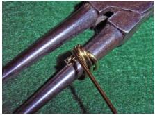
Then pull the string off the pliers, and try to push the nose of the pin through from the top. If you've done it properly, it won't go. So, holding the coils in your left hand, turn the pin anticlockwise to unwind the spring, pushing the pin as you go, until the top of the coils is at the right place on the pin.
