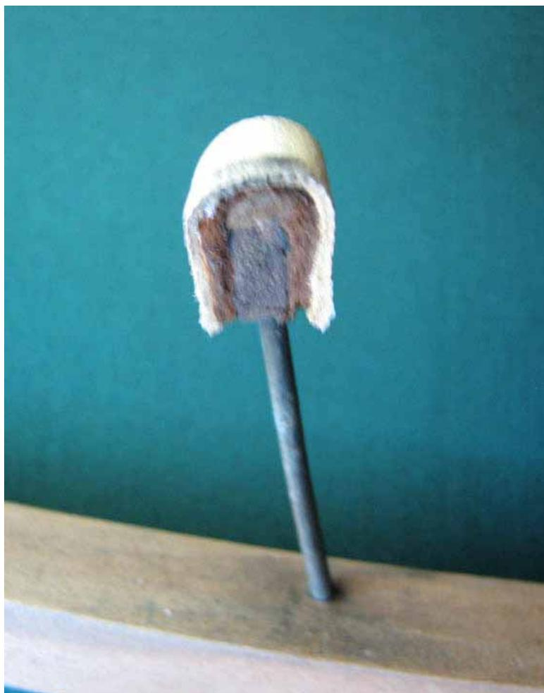
Replacing a hinge involved splitting the wood wedge and hammer butt away from the hammer shaft, and with a sharp knife slicing out the remaining leather hinge. Both wood faces should be clean of leather before the new hinge is inserted and the three pieces glued up. It is critical to line up the beveled end of the hammer with known good neighbors so that the hammer head will hit the intended pair of strings and not those above.
