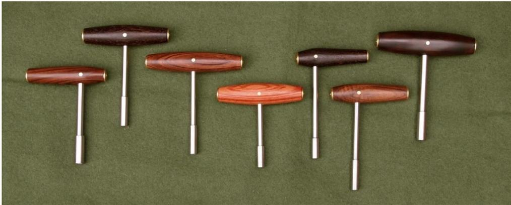
Obviously you need one, and it is important that it should be a good fit. Old instruments have hand-made flattened pins, and the hammer should grip the flats along the whole length (the ends do not matter). If the fit is sloppy, the corners of the pin will damage the socket, and be damaged themselves. There will also be backlash, which makes accurate tuning more difficult. On the other hand, if the socket is not big enough, it will grip only the tip of the pins, with damage as before.
